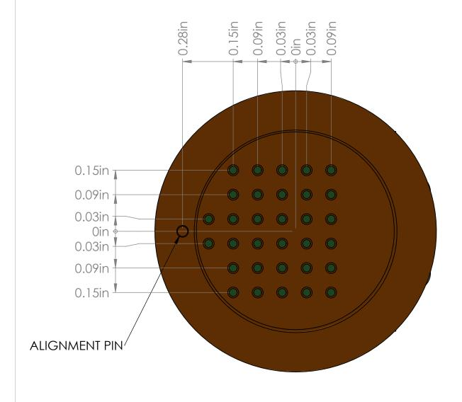
CONNECTOR SIDE OPPOSITE OF ALIGNMENT PIN
